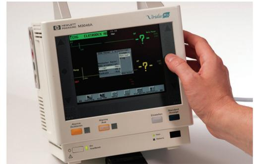
Stepless cursor control directly on the screen has only been possible with touch screens up to now, and was always a problem with dirty or greasy fingers. Sensofoil sensor controllers present a clean alternative, in particular for rough industrial conditions, because the screen surface remains clean and untouched.
