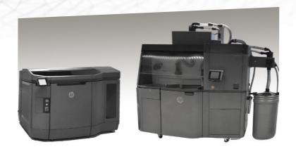
The innovative Multi Jet Fusion 3D printing process combines the strengths of the two well-known rapid prototyping processes – PolyJet and selective laser sintering (SLS) – and revolutionizing the world of 3D printing with its amazing performance: the Jet Fusion printers dispense 300 million drops of liquid per second with an accuracy of 21  $\mu$ m. The multifunctional Polyamide 12, known from the SLS process, serves as printing material.
