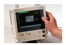
Stepless cursor control directly on the screen has only been possible with touch screens up to now, and was always a problem with dirty or greasy fingers. Sensofoil sensor controllers present a clean alternative, in particular for rough industrial conditions, because the screen surface remains clean and untouched.
