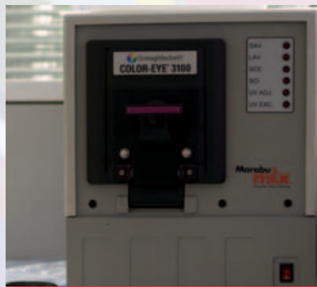
Better accuracy than the human eye: the colorimeter Colour Eye 3100
