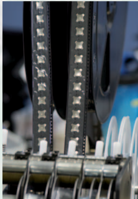
Snap discs run on a wheel and are applied to the designated position
