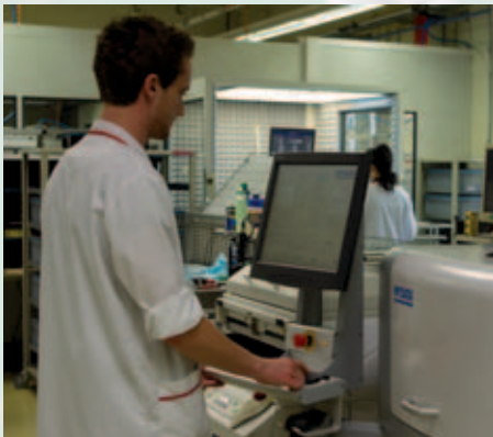
The soldering paste printer by MyData is the acquisition of machinery
