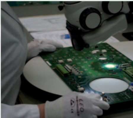
Visual inspections of the assembled components are carried out with great attention to detail
